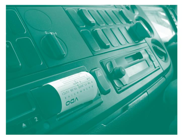
Digital tachographs work by storing digital data on the driver and vehicle in their own memory and separately on a driver's smart card. Transport undertakings must periodically download this data from the digital tachograph (known as the Vehicle Unit or VU) every 56 days and from driver cards every 28 days and analyse the information to ensure that the rules have been complied with.
